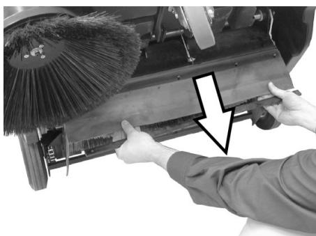
→ Readjust the sealing strips pushing them downward into the slot.
