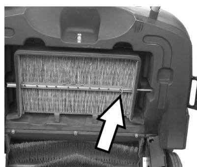
→ Remove the securing splint of the vibrator bar.
